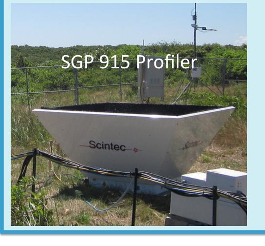
The ARM Program's 915 Radar Wind Profilers have recently been reconfigured to add modes at vertical incidence, sampling profiles up to 15 km in height. In zenith mode, the radars are sometimes referred to informally as UHF ARM Zenith Radars, or UAZRs. They have 9° beamwidths, 200 m gate spacing and time resolution of 5 s. The two alternating zenith modes differ in pulse length, Nyquist velocity and maximum
