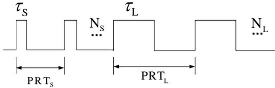
**Fig. 1 Combined-pulses transmission mode in diagram**
