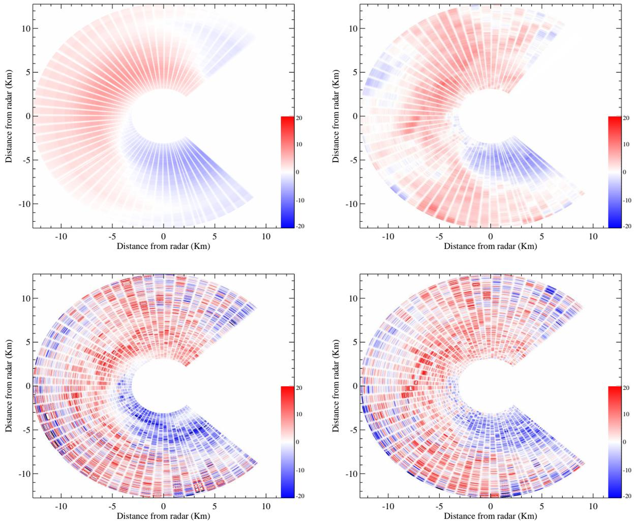
Figure 2: Baseline wind measurements at an elevation of 20 degrees. Clockwise from top left. (a) - VAD-like variational retrievals of baseline wind. (b) - DBS retrievals (c) - Spaced antenna retrievals using the FSA algorithm. (d) - Spaced-antenna retrievals using the G-SZL algorithm. Positive velocities indicate clockwise motion.
