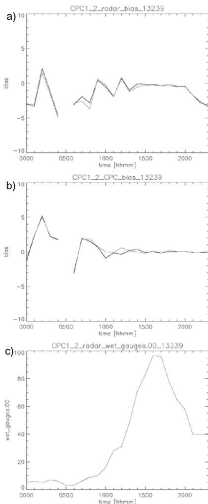
Fig. 6 Evolution of the hourly bias between radar and rain gauge measurements for the development (black line) and operational (grey line) products: a) radar only data, b) radar data adjusted with rain gauges (independent set), c) number of wet rain gauges during the hour.
