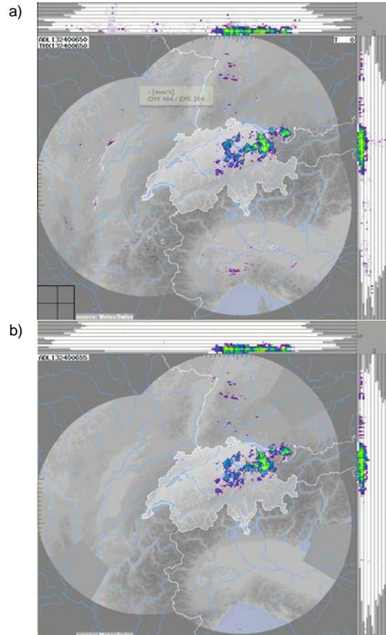
Fig. 5 Example of QPE product: a) Operational, b) Produced by development chain
