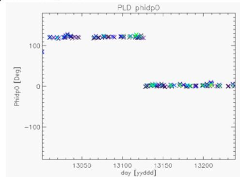
Fig. 2 Dole  $\phi_{dp}$  offset in 2013. Bluish colors correspond to lower elevations. The offset has been software corrected from day 120.
