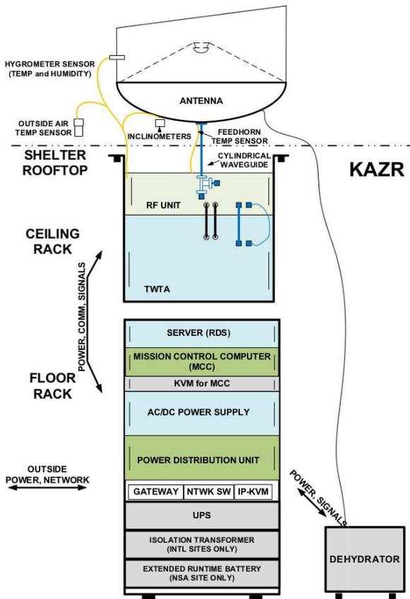
Figure 3: Illustration of the KAZR sub-system assembly.
