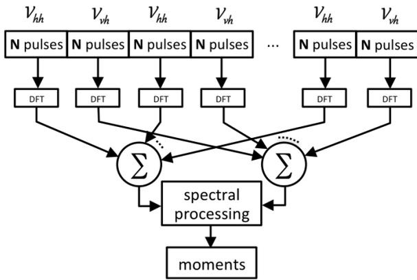
Figure 6: Diagram illustrating the processing of co-polar and cross-polar returns to estimate the moments.
