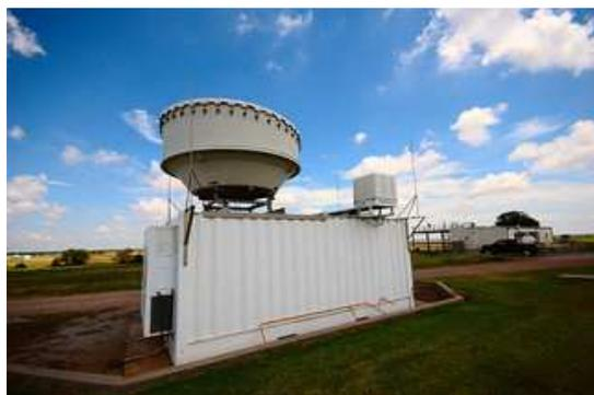
Figure 1: Photograph of KAZR deployed at ARM's Southern Great Plains site in northern Oklahoma.
