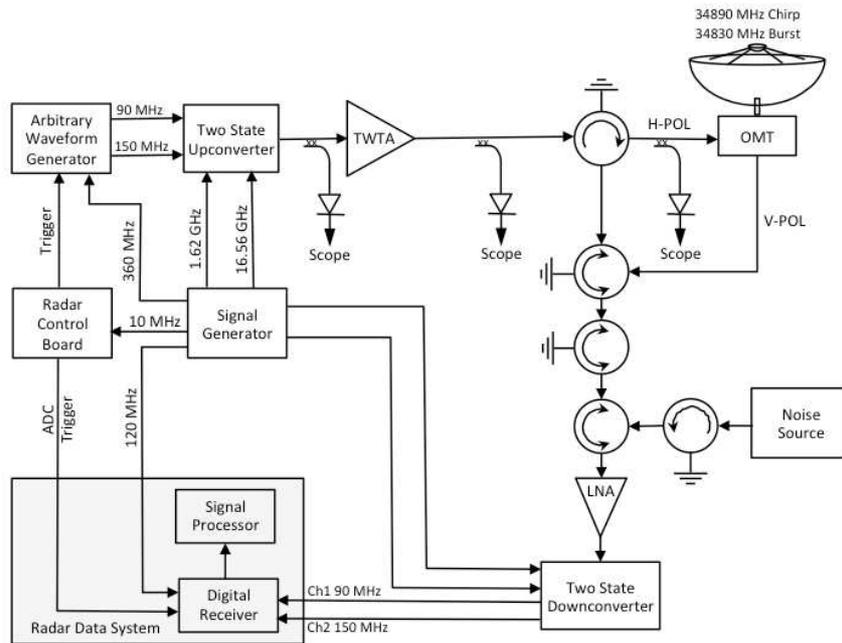
Figure 2: A simplified block diagram of KAZR.
