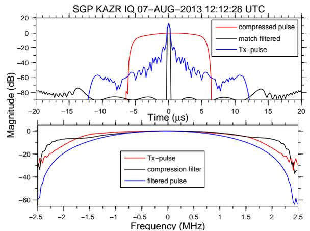
Figure 4: Use of  $T_2 = 12 \mu s$  pulse compression waveform at Manus and the response of the compression filter.
