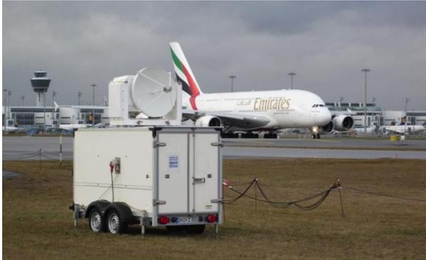
**Fig. 1** Scanning MIRA-36 mounted on a trailer at the Munich airport with antenna pointing towards the gliding path (elevation=5°)
