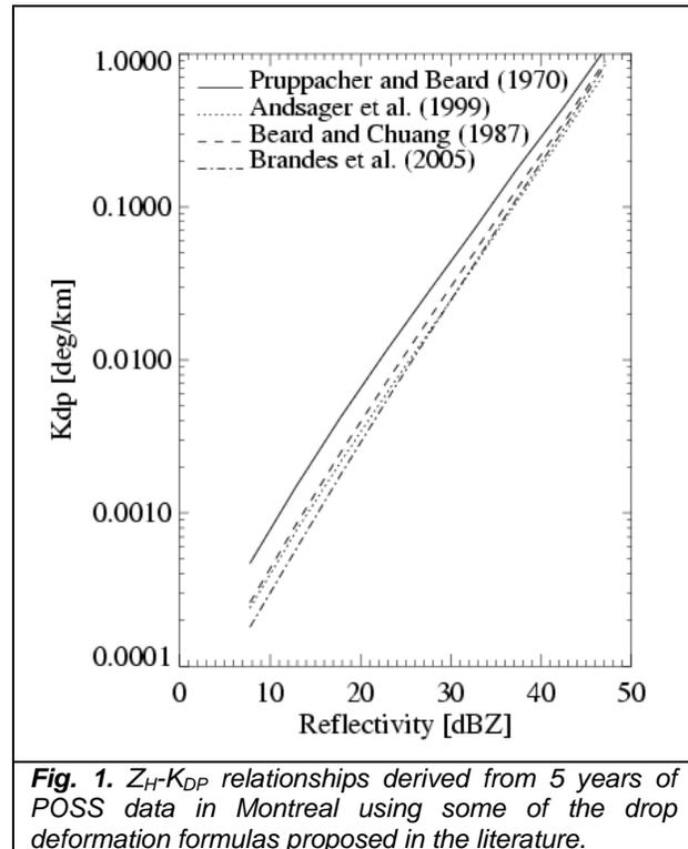
**Fig. 1.**  $Z_H$ - $K_{DP}$  relationships derived from 5 years of POSS data in Montreal using some of the drop deformation formulas proposed in the literature.
