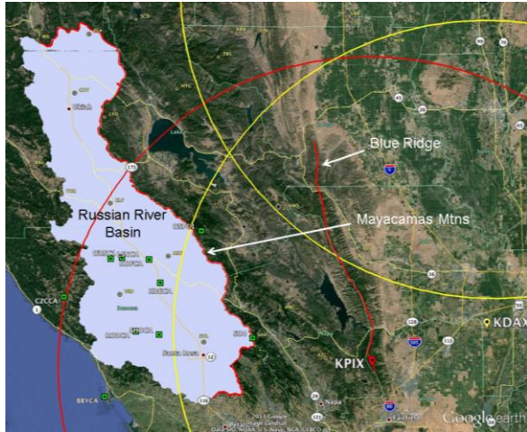
Figure 2. Radar and gauge locations surrounding the Russian River basin. Analysis gauges are yellow and validation gauges are green.
