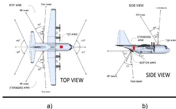
Figure 1: Position of the four AESA's on the NSF/NCAR C-130: a) top view and b) side view
