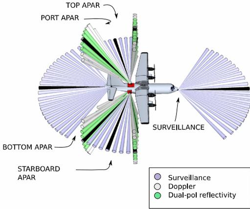
Figure 2: Illustration of the proposed radar scanning modes on the NSF/NCAR C-130. Note top antenna is displaced to better illustrate Doppler scanning.
