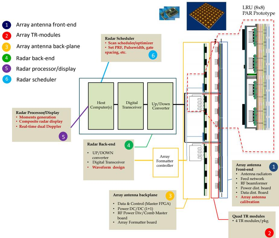
Figure 3: Simplified block diagram of APAR architecture. Subsystems 1-3 reside outside the fuselage, enclosed by a fairing/radome; the rest of the system resides in the cabin.
