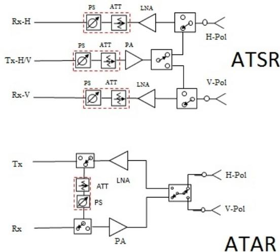
Figure 4: Simplified block diagram of dual-pol TR module architectures, ATSR and ATAR
