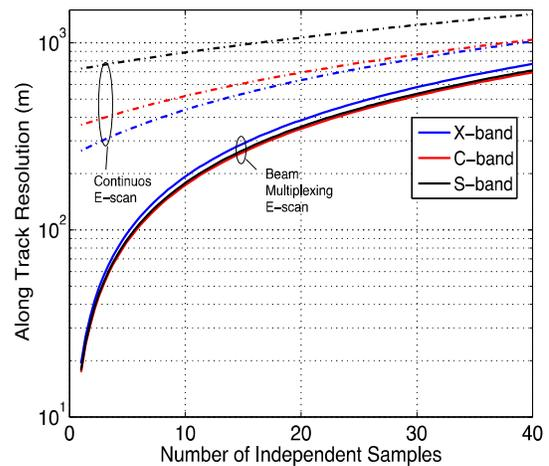
Figure 6: Along-track resolution as a function of the number of independent samples for S-band, C-band, and X-band. Scanning range of 90°, beam overlapped factor of 35%, flight speed of 120 m/s, and PRF of 2000Hz.
