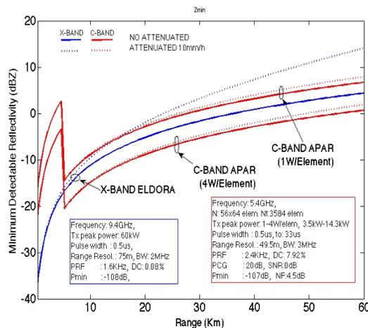
Figure 5: Minimum detectable reflectivity vs. range for ELDORA, APAR with 4W/element transmit power and APAR with 1W/element transmit power
