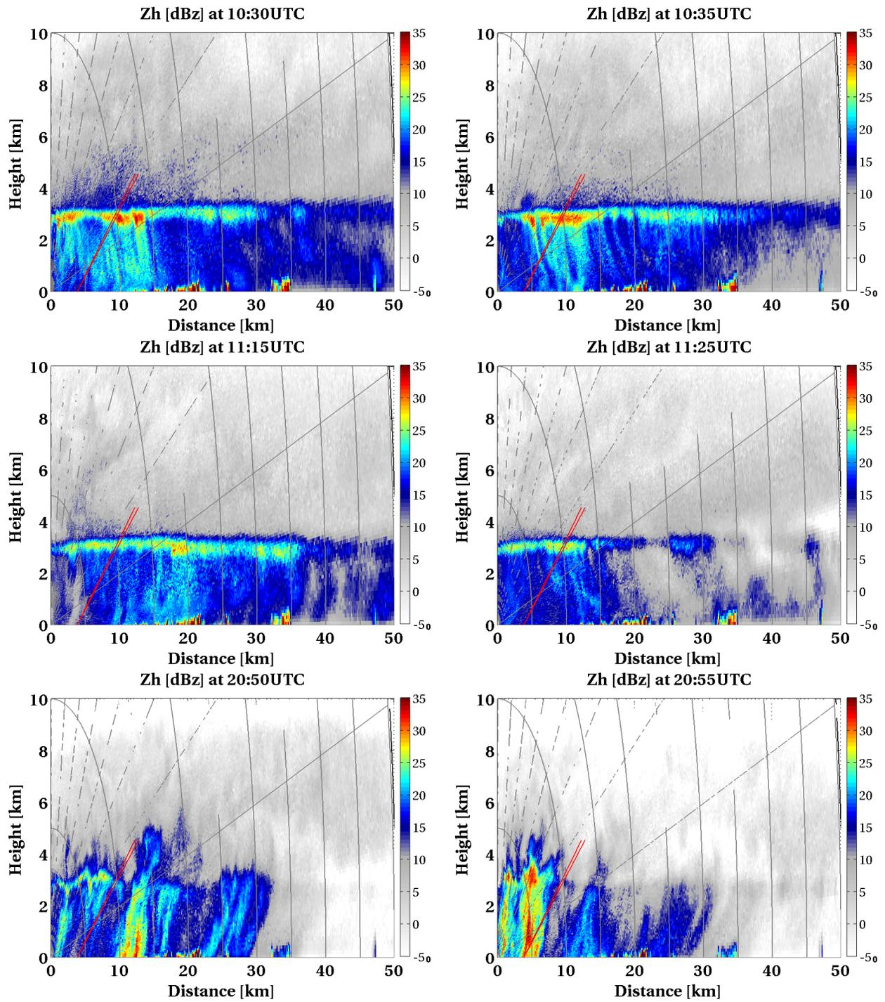
Figure 3: JuXPol radar RHI sequence at same ADMIRARI's azimuth. Red cone represent the instantaneous radiometer FOV.
