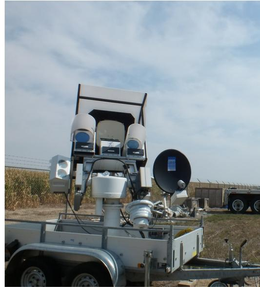
Figure 1: ADMIRARI radiometer at Jülich Research Center. Note the auxiliary active sensors MRR (right) and cloud lidar (left).
