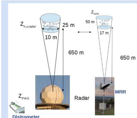
Concept to monitor absolute calibration: relate farfield range bin from birdbath scan to disdrometer: Assumption: temporal and spatial homogeneity of the precipitation process MRR is used to verify the assumptions.
