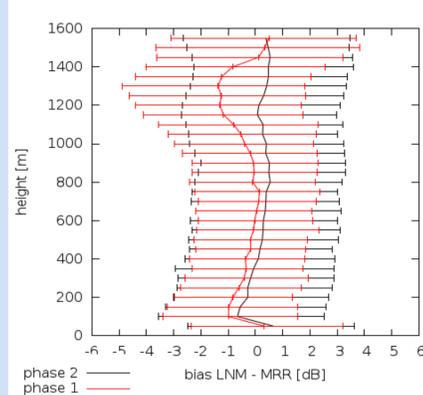
The bias of MRR Z measurement relative to the disdrometer data as a function of measurement height. The bias profile considers simple time correction to relate disdrometer with elevated radar measurements.
