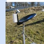
Vertical pointing MRR with a range resolution of 50 m. The MRR is a FM-CW radar and operates at 24 GHz. Standard MRR signal processing for rain is used, including path attenuation correction and Mie-to-Rayleigh scattering adjustment. Vertical air motion related to mountain flow is neglected at the reference height of 650 m above site.
