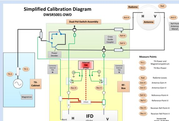
Simplified calibration diagram illustrating the transmit and receive path of the DWD radar system, including relevant elements which have to be characterized for an accurate engineering calibration. Z of the H and V channel should be within +/- 1 dB.
