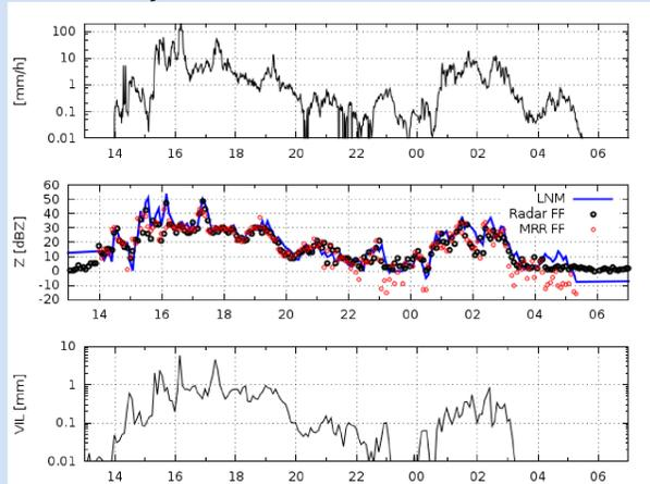
Timeseries of precipitation rate (upper panel, disdrometer data), a comparison of the reflectivity factor Z based on radar and MRR (650 above ground, in the farfield (FF) of the radar antenna, and Z computed from the DSD measured by the disdrometer (middle panel), and VIL computed from the birdbath scan (lower panel). Z agrees particularly well for 15 < z < 30 dBZ, stratiform conditions. 55.9 mm precipitation was measured during this event.
