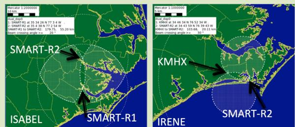
Fig. 2. Dual-Doppler lobes ( $30^\circ$  cross-beam angle; white shading) shown for each SMART-R deployment to Isabel (a) and Irene (b). SMART-R2 is used as the origin in Isabel and KMHX in Irene. Radar positions are shown via the black arrows.
