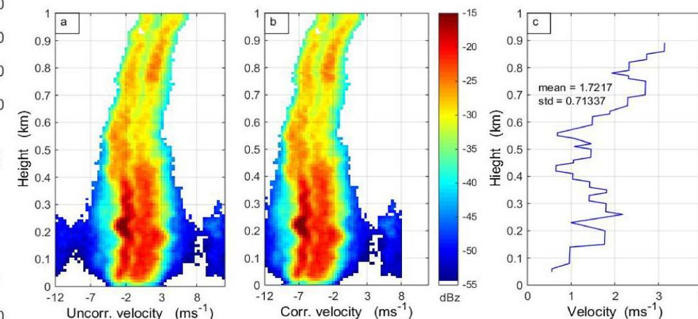
Fig. 4 Corrected (b) and uncorrected (c) spectrogram, and vertical air velocity profile at 20:06:42 UTC, 22 May 2012 in Key West, Florida.
