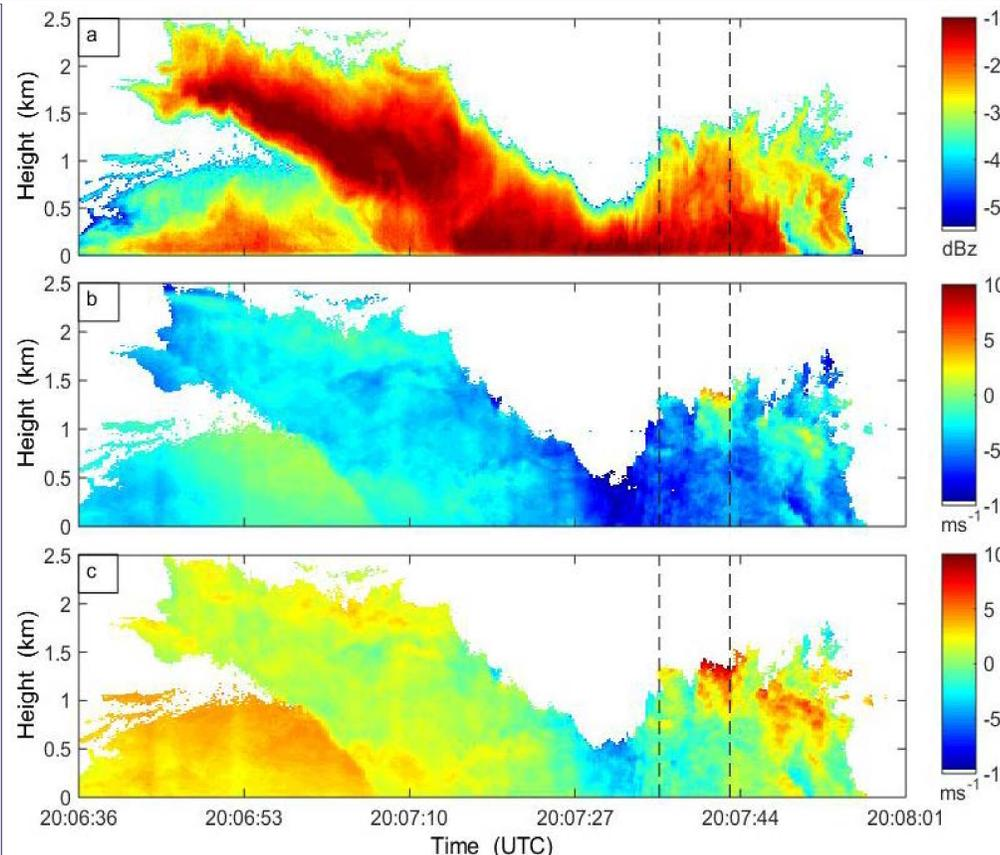
Fig. 2 Reflectivity factor (a), corrected Doppler velocity (b) and uncorrected Doppler velocity (c), 05/22/2012, Key West
