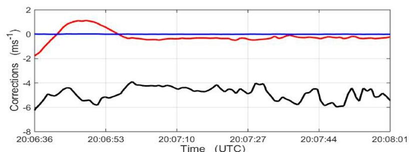
Fig. 1 Correction terms related to aircraft motion (black), horizontal wind (red) and apparent velocity (blue).
