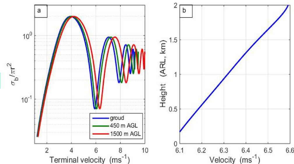
Fig. 3 (a) Simulated spectra with or w/o air-density correction at ground, 450 m and 1500 m AGL, 22 May 2012 in Key West, Florida; (b) air-density-corrected terminal speed profile ARL for 1.69 mm raindrop.
