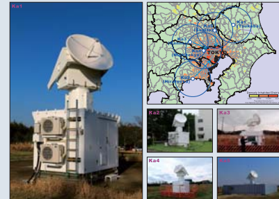
Figure 1. Photos of five Ka-band cloud radars and their distributions on a map around Tokyo (upper right). Blue circles indicate the observation ranges ( r=30 km) of each radar. Colored areas indicate densely inhabited districts. Some radars are planned to move to near Tokyo.
