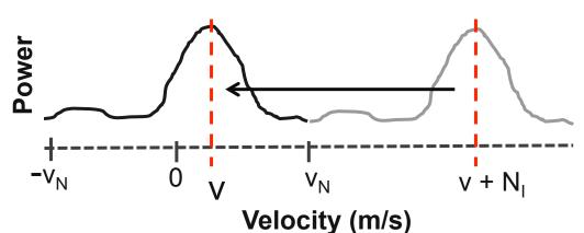
Various algorithms have been designed to unfold or dealias the measured velocities to determine the true atmospheric velocities. Most algorithms are designed to unfold velocities from a single scan type (PPI, RHI or vertical pointing) and perform best at specific radar frequencies and Nyquist velocities. Here we present two novel algorithms which can unfold velocities from data collected at various wavelengths, Nyquist velocities and scan types.
