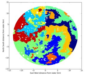
Raw and segmented velocities from the ARM CSAPR radar in the SGP. Data is from the first 150 gates of a PPI scan at the highest elevation (42°) collected at 10:47 UTC on May 20, 2011
