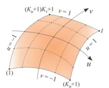
Generalized curved quadrilateral patch for MoM-SIE scattering modeling of melting hail. Model B is meshed with 1360 quadrilateral elements and 5440 unknown coefficients of current expansion.
