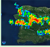
Figure 10: Reflectivity PPI scan from NEXRAD. Waterspout is not detected.
