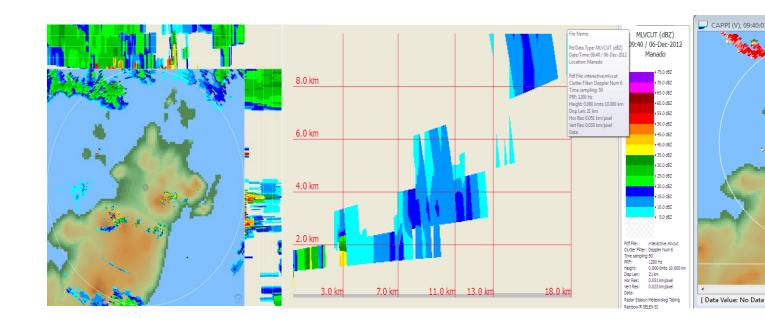
This eruption is the first weather radar analysis in Indoneisa for Vulcanic ash detection. For do analyze and recognize the ash volcano echo, do Cross section to make sure Ash Volcano Signature. Cross Section from the Ash Volcano suspect, from the data its have different signature if we compare with precipitation echo. Its low intensity without developed phase like precipitation cloud For look trajectory we can use the velocity data to know the direction of ash volcano movement
