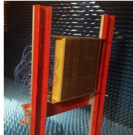
Fig. 3: 64 elements array in NF chamber.
