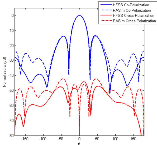
Fig. 4: principal plane cut of 4x4 array simulation by HFSS and PASim Version 1.
