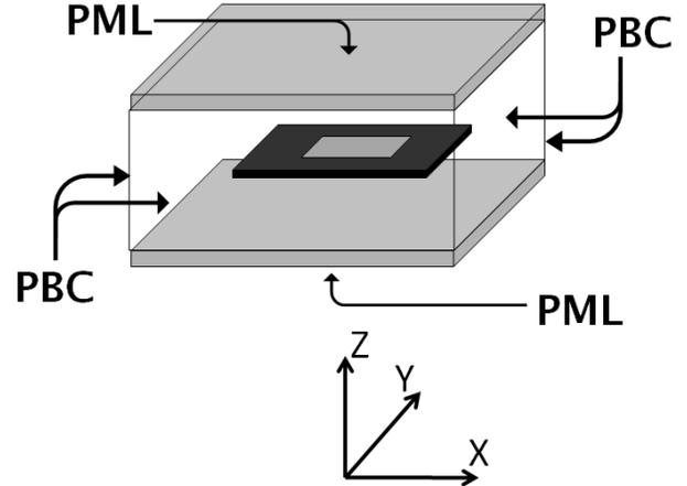
Fig. 1: The model of one unit cell in the phased Array.
