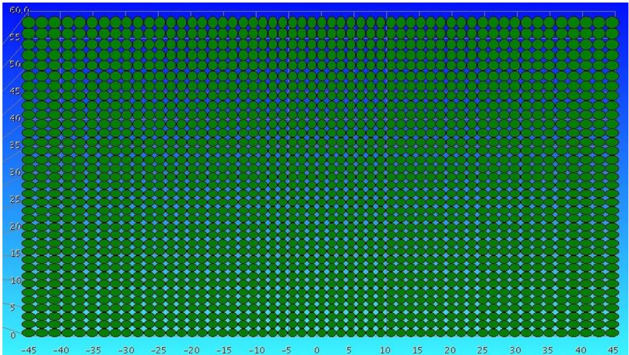
Fig. 3. RCI client ADAPTS beam map display for the full azimuthal extent of the fast surveillance, or detection, VCP. Green ovals represent all of the beam positions in the VCP. The shape and size of the ovals represent the beam coverage. Note non-overlapping beams and lack of gaps between elevations.
