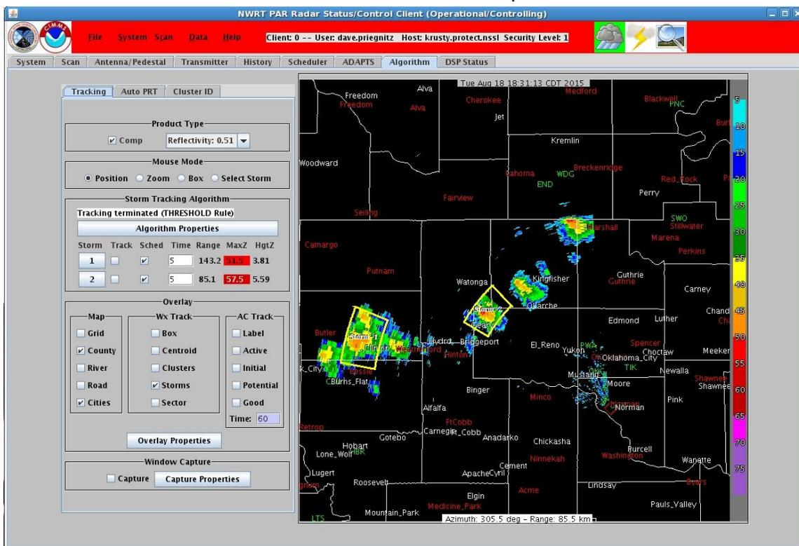
Fig. 2: RCI client algorithm display window containing 0.5° PPI reflectivity display with storm boxes overlaid.
