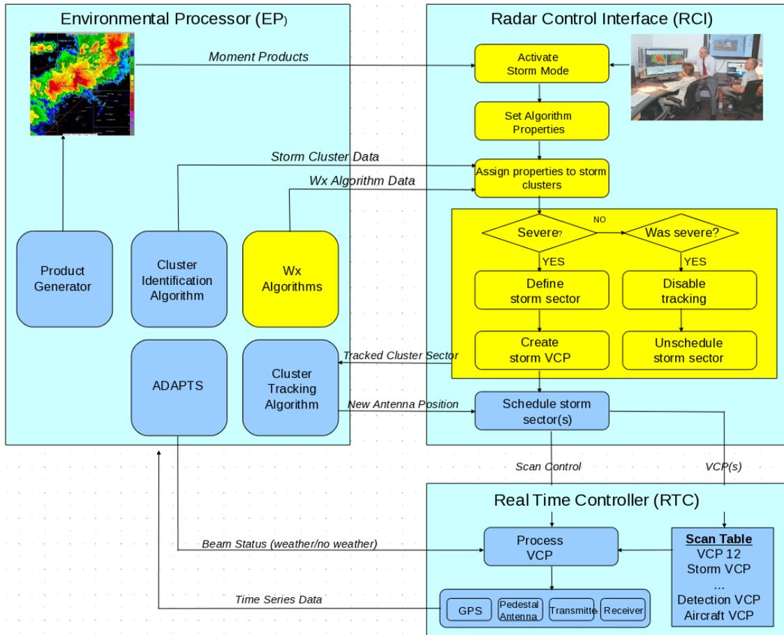
Fig. 1. A functional diagram of the adaptive scanning process at the NWRT PAR.
