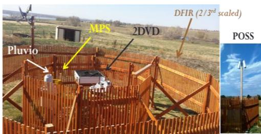
Fig. 1: The MPS, 2DVD and Pluvio inside the double wind fence, and the newly installed POSS.
