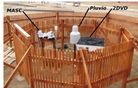
Figure 2: Instrumentation installed at the Easton Airport site during the November 2014 – April 2015 period of MASCRA project operations.
