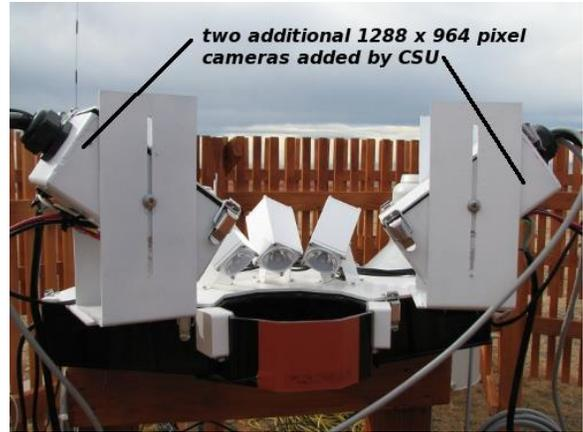
Figure 4: Two additional downward-looking cameras added to the CSU MASC.
