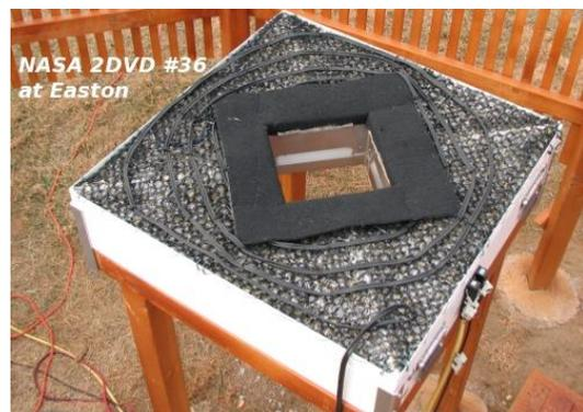
Figure 5a (top): 2DVD schematic diagram (from Schönhuber, 2008). 5b (bottom): 2DVD as installed at the Easton site.
