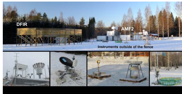
Figure 4: Instruments install in BAEC test site. Note that Pluvio 2 200 was inside the DFIR. We used it as reference.
