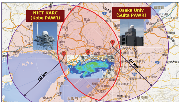
Fig.3. Observation range of Kobe and Suita PAWRs and dual-Doppler observation area. The colored area over the Osaka-bay shows convective echo measured by dual PAWRs.
