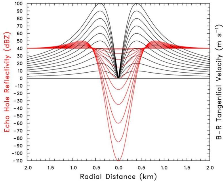
**FIG. A1.** Profiles of the reflectivity hole and surrounding reflectivity ring (red) across the center of Tornado 4 associated with overlaid Burgers–Rott tangential velocity profiles (black). The uniform reflectivity curve at 40 dBZ corresponds to the uniform tangential velocity curve at  $0 \text{ m s}^{-1}$ . The other reflectivity curves correspond to tangential velocity curves represented by peak values ranging from 10 to  $100 \text{ m s}^{-1}$  at intervals of  $10 \text{ m s}^{-1}$ .
