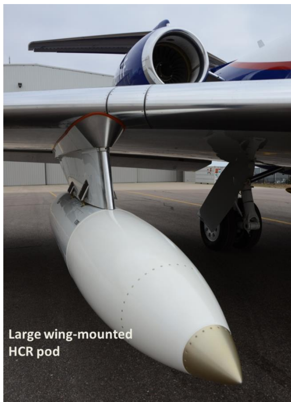
Fig 1. Photo of the HCR pod mounted on the HIAPER aircraft's wing.
