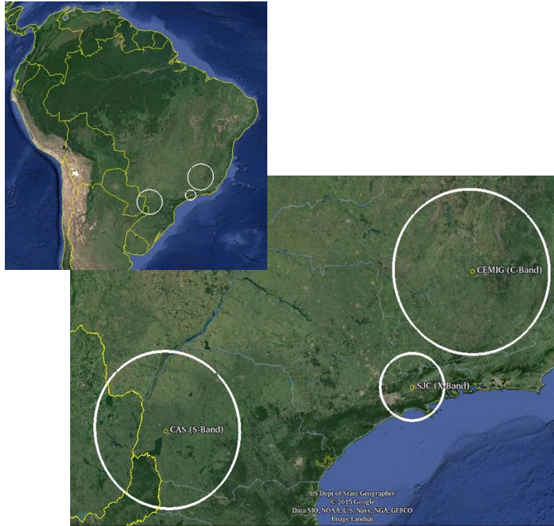
Figure 1: Radar site and coverage area. Range circles are 240 km, 100km and 250 km for the Cascavel (CAS), São José dos Campos (SJC) and Morro do Elefante (CEMIG) radars, respectively.
