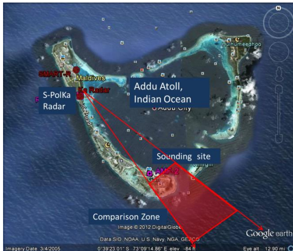
Fig. 5. The Addu Atoll with the locations of the S-PolKa radar, DOE sounding site and a sketch of the region for radar humidity retrievals compared to the sounding (red shading).
