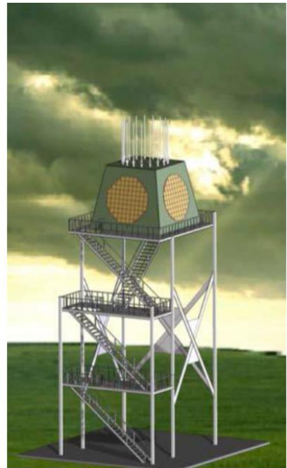
Figure 1. Notional parameters of Terminal MPAR. The radar would consist of 4 planar faces and would typically be located on airport property.
