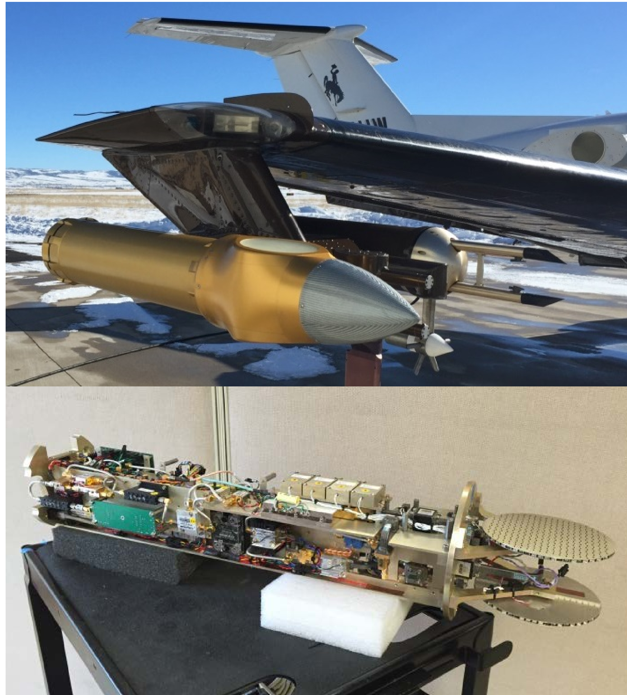
Figure 2. The University of Wyoming Ka-Band Precipitation Radar (KPR) is a compact, dual-beam Doppler radar that operates from a standard PMS (Particle Measurement Systems) probe canister.
