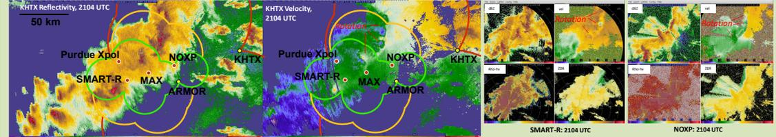
Best theoretical dual-Doppler lobes between VSE radars (not accounting for blockage, attenuation, etc.), with baselines: < 25 km (green), 25-40km (yellow), and +40km (red). Mobile radars with available data from the same time as the KTHX image to the left. (0.8 or 0.5-degree elevation angle).
