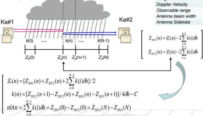
This method provides the both total path attenuation and the attenuation efficient at each range. And equivalent radar reflectivity can be retrieved directly by combining two measured reflectivity profiles without any a priori knowledge of the attenuation characteristics along the path. Hence it is suitable to measure melting layer, which has large variety of attenuation in small range.
