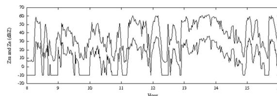
Comparison of radar reflectivity from DKR and Parsivel data on 26 Nov. 2013. Upper curve is from DKR and lower is from Parsivel. Curve from DKR is biased with 40 dB to avoid overlapping of the two curves. (Prof. Nakamura)
