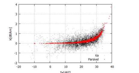
k and corrected Ze of dual-Ka method shows the good agreement with theoretical k-Ze relationship from DSD of Parsivel in case of rain.
