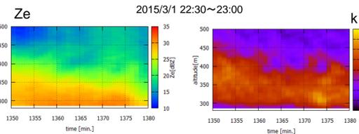
As the height of melting layer decreases from 400m high to below 300m high during 30 minutes.
