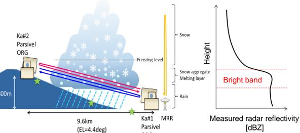
★ Three G-PIIMS, abbreviation for "Ground-based Particle Image and Mass Measurement System", which was newly developed for this experiment by Dr. Suzuki, Yamaguchi University
