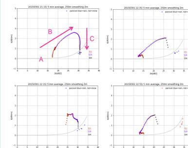
the variation of k-Ze. Both k and Ze in minor area(A) is above the melting layer where the particle is solid. As the ratio of number of melting particle and melting ratio in a particle itself increases, the k and Ze are also increasing(B). After going over a peak of k, Ze is almost constant but the k rapidly decline (C) and it will conform to the k-Ze relationship of rain of DSD at the ground at the end(D).
