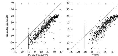
Scattergram of the radar reflectivity derived from DKR and Parsivel data. Left is with Mie scattering calculation in Parsivel data, and right is with Rayleigh scattering calculation. The data at -10 dBZ in Parsivel represent non-available data. (Prof. Nakamura)
