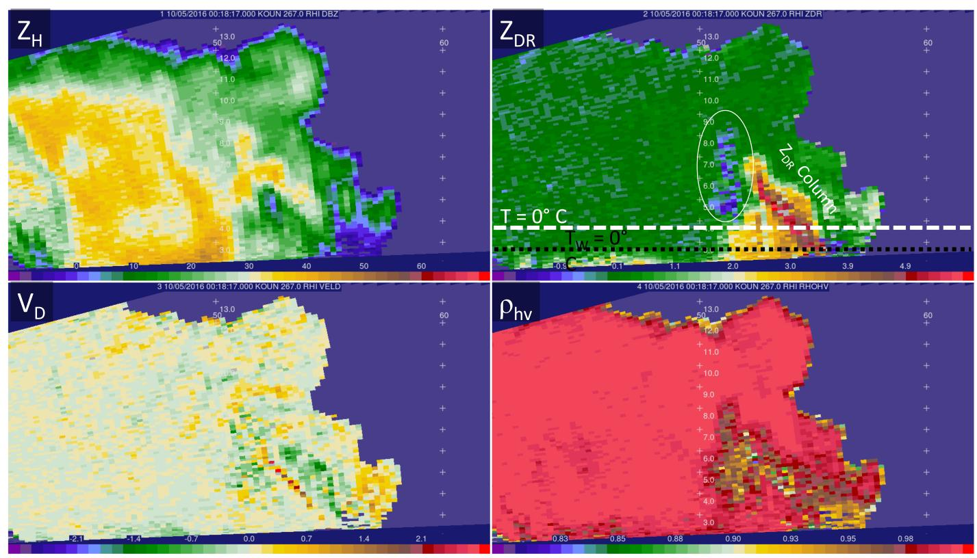
KOUN (in central OK) has been used to collect RHIs for better examining polarimetric characteristics of very large hail and hail growth. Time series data collection enables spectral processing and allows us to examine nonstandard products (e.g., differential Doppler velocity,  $V_D$ ).  $Z_{DR} < -1$  dB is observed near/above the  $Z_{DR}$  column in (above) an October 2016 supercell and (below) a June 2017 supercell (depolarization ratio, DR, is shown).
