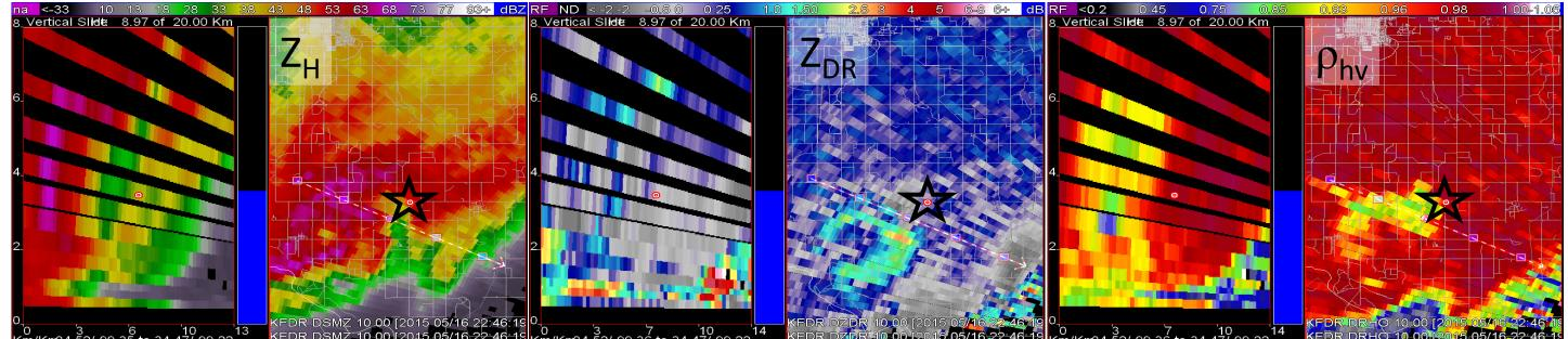
Vertical cross-sections (left side of each panel) and 10.0° elevation angle PPI (right side of each panel). Very large hail fell along the northeast side of the weak echo region, northeast of a crescent-shaped  $Z_{DR}$  column or  $Z_{DR}$  ring. The north side of the  $Z_{DR}$  column was characterized by  $\rho_{hv}$  as low was 0.85.  $Z_{DR}$  as low as -1.5 dB was located immediately northeast of the  $Z_{DR}$  column.
