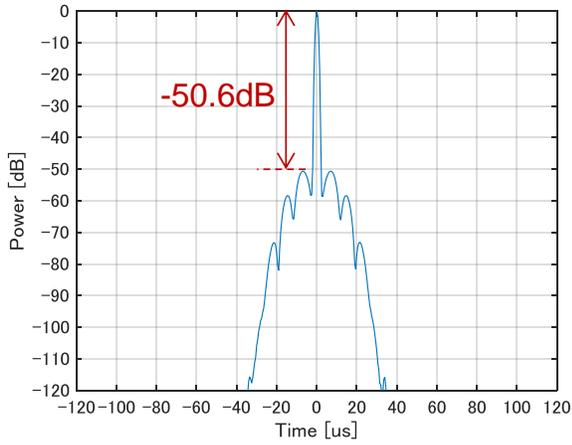
**Fig. 3: Pulse Compressed Waveform (LFM T=36µs, Simulated Result)**
