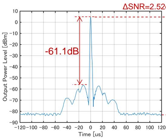
**Fig. 11: Pulse Compressed Waveform (LFM T=72µs, Measured Result)**
