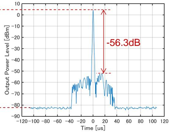
**Fig. 13: Pulse Compressed Waveform (NLFM T=36µs, Measured Result)**
