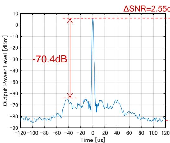
**Fig. 12: Pulse Compressed Waveform (LFM T=108µs, Measured Result)**
