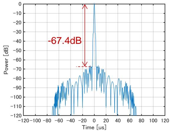
**Fig. 7: Pulse Compressed Waveform (NLFM T=72µs, Simulated Result)**
