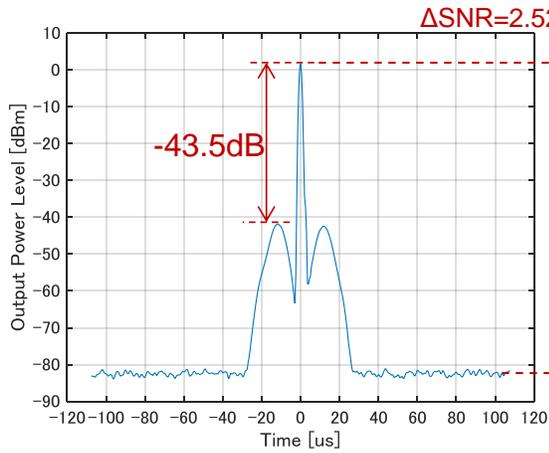
**Fig. 10: Pulse Compressed Waveform (LFM T=36µs, Measured Result)**
