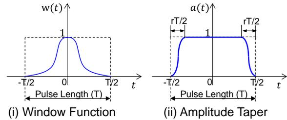
Fig. 2: Schematic Drawings of Window Function and Amplitude Taper
