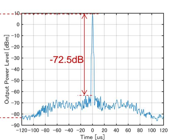
**Fig. 15: Pulse Compressed Waveform (NLFM T=108µs, Measured Result)**
