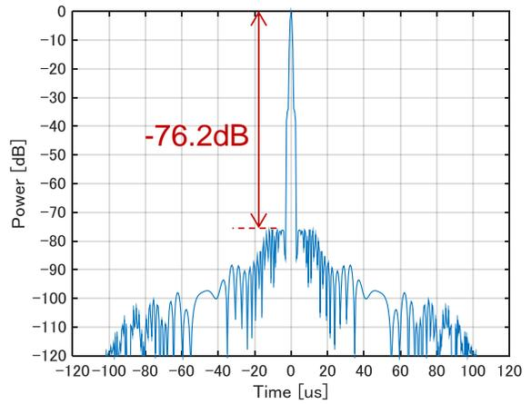
**Fig. 8: Pulse Compressed Waveform (NLFM T=108µs, Simulated Result)**
