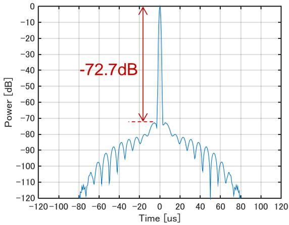
**Fig. 5: Pulse Compressed Waveform (LFM T=108µs, Simulated Result)**
