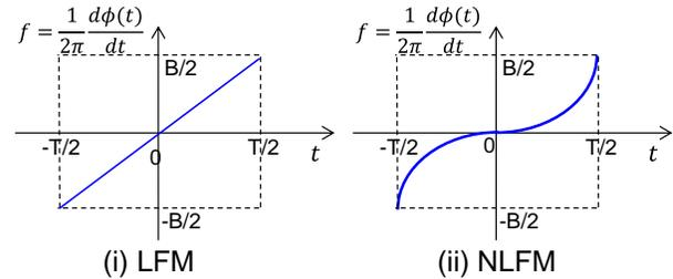
Fig. 1: Schematic Drawings of LFM and NLFM
