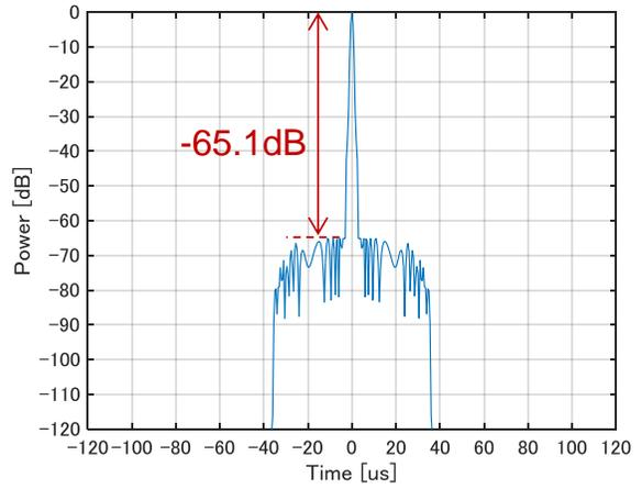
**Fig. 6: Pulse Compressed Waveform (NLFM T=36µs, Simulated Result)**
