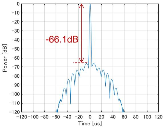
**Fig. 4: Pulse Compressed Waveform (LFM T=72µs, Simulated Result)**
