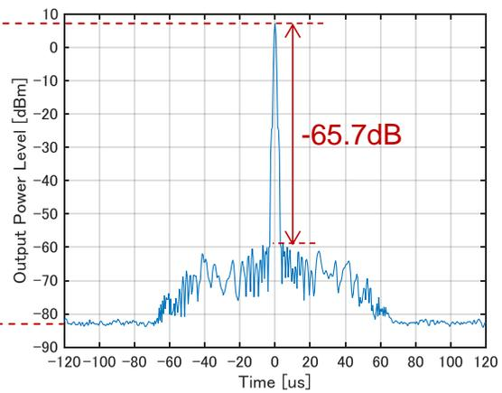
**Fig. 14: Pulse Compressed Waveform (NLFM T=72µs, Measured Result)**
