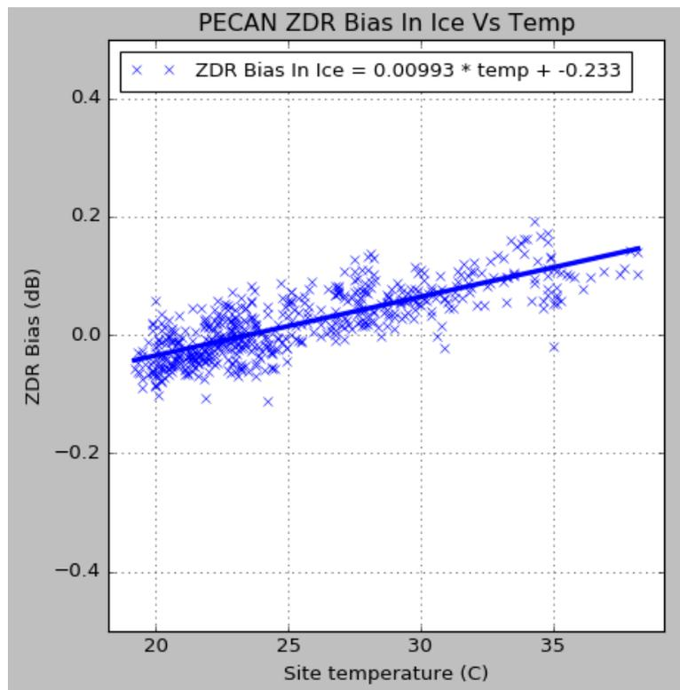
Figure 11. Regression plot of observed ZDR bias (from the 15<sup>th</sup> percentile) vs the site temperature, for PECAN from June 16 to July 16 2015.
