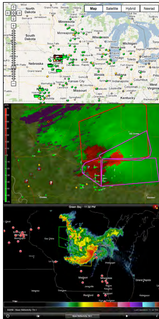
Figure 5: Spotter Network integrates effortlessly into many mapping and weather program by providing various data feed formats (XML, TXT, KML, etc.) available for use in third party products such as Google Maps® (TOP), GRLevel3 & GR2Analyst (MIDDLE), and Radar Scope for iPhone and iPad (BOTTOM), which can display live tracking position icons of mobile or stationary storm spotters along with personal information if made available by the individual.
