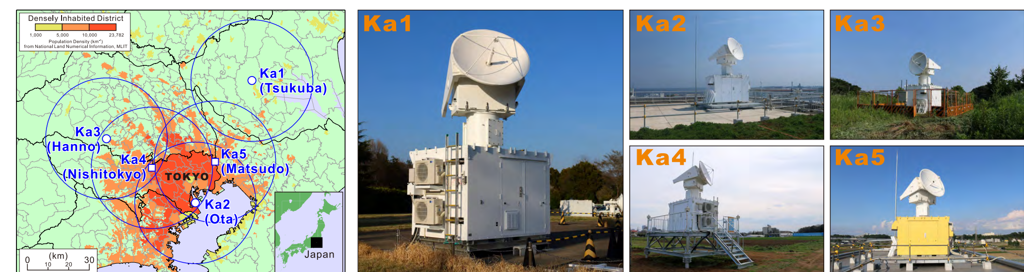
Distributions of five Ka-band cloud radars (left) and their photos (right). Blue circles indicate the observation ranges ( r=30 km) of each radar. The radars indicated by open circles are dual-polarization radars, while open squares indicate single polarization radars.
