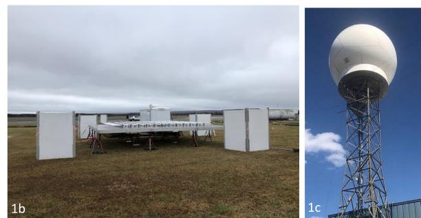
Fig. 1b shows the S-band profiler radar. Fig. 1c shows the C-Band ARMOR radar. Table 1 on the right side presents some important technical specifications and operating parameters of both instruments. Table 2 below shows the precise deployment locations of the instruments.
