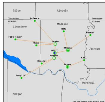
Schematic showing the 11 sensors and receiving station that comprise the NALMA network.
