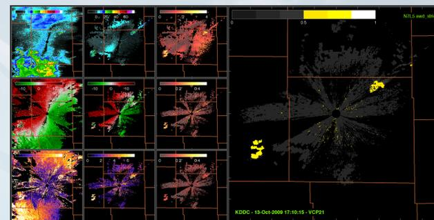
Two wind farms, one located 40 km southwest while the other lies 25 km northeast of the KDDC radar site were successfully identified. Note the similar values in reflectivity, velocity and spectrum width for the precipitation at the southwestern region that would be nearly impossible to identify without a temporal history of data.
