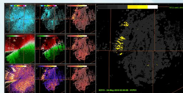
The wind farm just west of the KDYX radar was detected. Streak-like echoes are due to multipath propagation but the texture signatures of the wind turbine clutter do not change, which make the detection viable.
