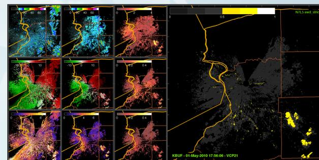
Several wind farms southeast of the radar have been detected using the automated wind turbine identification algorithm.
