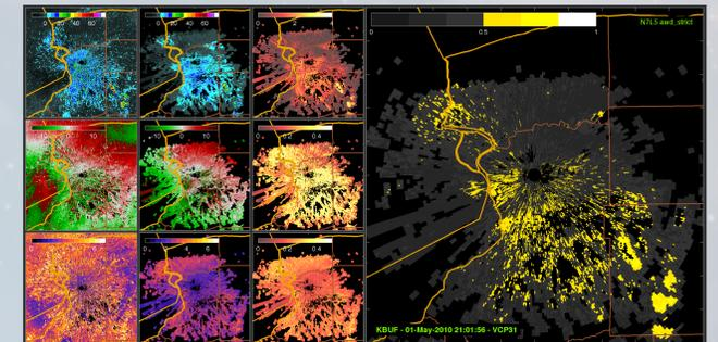
Low PRF that causes velocity measurements to alias and induces positive bias on the spectrum width estimate could consequently cause large amount of false detections. In addition, lower PRF's are usually accompanied with lower number of pulses per radial, which introduces a positive bias on  $W_v$  and, thus,  $R_w$ . This would cause four out of six textures to be misrepresented and result in false detections.
