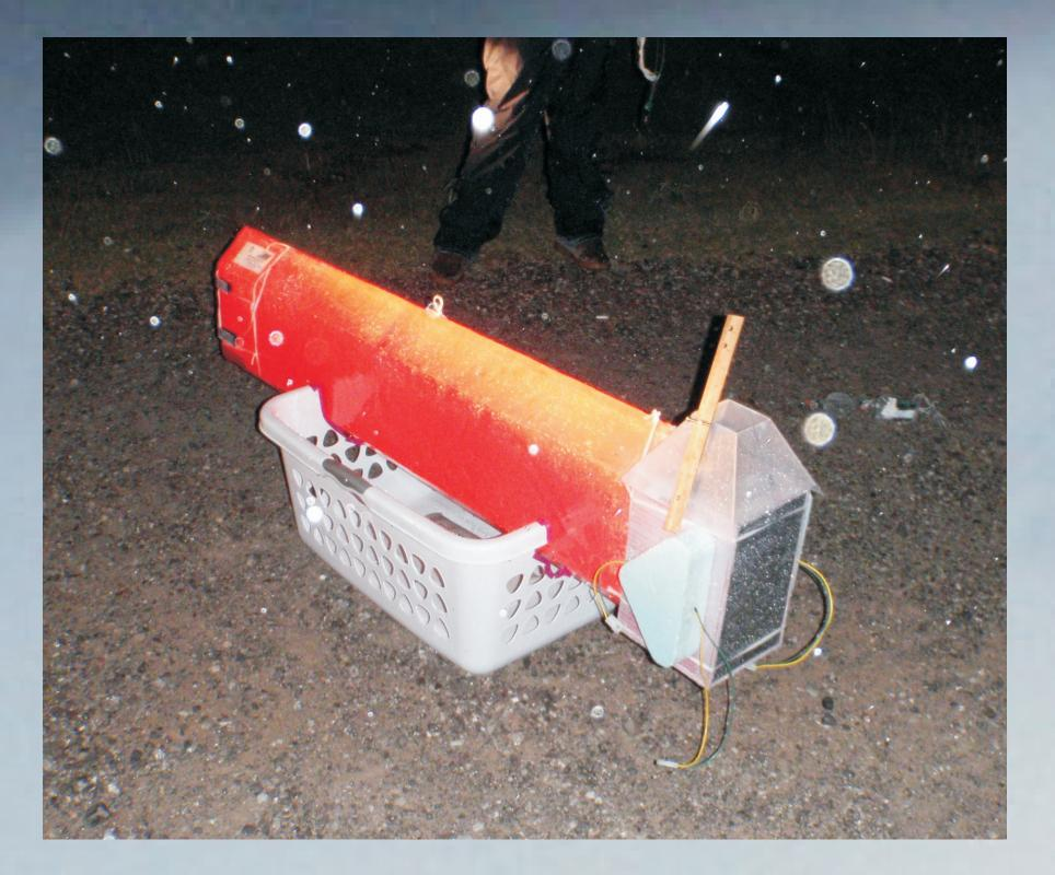
NSSL and CIMMS are developing the high-definition videosonde for several applications: ground truth for hydrometeor classification schemes of polarimetric radars, improving microphysical parameterizations in numerical cloud models, improving understanding of hydrometeor processing of chemical species, and improving understanding of thunderstorm electrification and lightning production.
