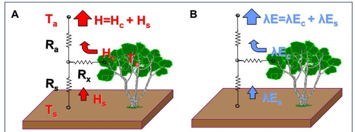
Figure 2: A simple schematic representation of the Two-Source Energy Balance Model. Panel A shows the sensible heat flux while Panel B shows the latent heat flux.
