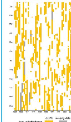
Figure 3. Streamflow deficiency periods below the varying threshold level Q70
