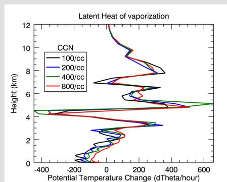
Deep convective clouds produce less surface evaporation in simulations with higher aerosol concentrations. This is can likely be attributed to the significantly larger rain drop sizes that exist in these environments (seen before in Storer et al. 2010).
