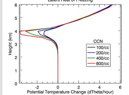
Simulations with higher aerosol concentration have deep convective storms that contain more ice mass. The increase in ice mass is associated with an increase in melting that occurs though a deeper layer (Not shown are the larger hail sizes that exist in polluted storms – hence the hail will fall farther and melt though a deeper layer.) Stronger cooling can be seen near the freezing level in simulations with higher aerosol concentrations which corresponds to this increase in melting.
