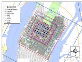
Figure 1. The horizontal bounds of the model domains for each of the model participants. The grid of red and blue markers in the center represent locations of 30-min average tracer measurements.
