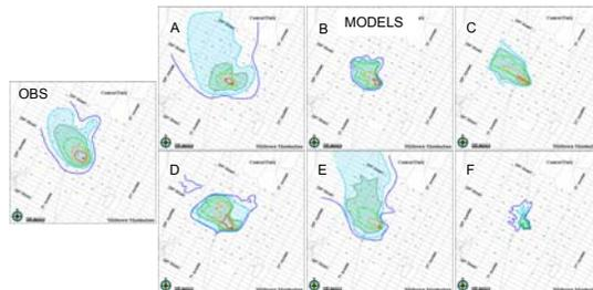
Figure 5. Near-surface tracer plume from the six models compared with measurements. Half-hour average concentrations coincident with a tracer release period (same as Figure 6). Wind speeds were moderate and the wind speed was steady from the south.
