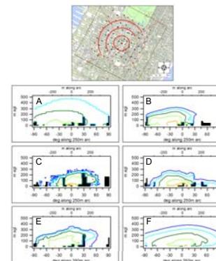
Figure 6. Vertical mixing of tracer on a half-cylinder 250m from the source. (Shown as the smallest radius arc in the top panel.) Half-hour average concentrations coincident with a tracer release period (same as Figure 5).
