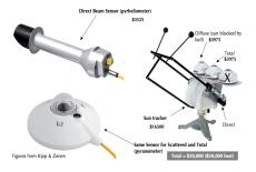
First-class instruments for measuring direct beam, total horizontal and diffuse horizontal irradiance plus the tracker for direct bean and diffuse measurements are illustrated in this figure along with last year's prices
