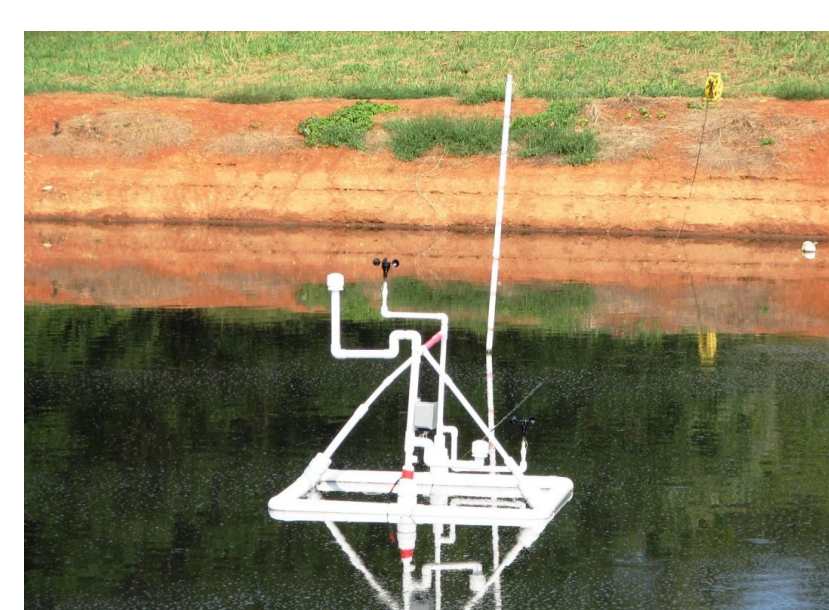
Figure 1. Floating raft containing instrumentation on lagoon surface
