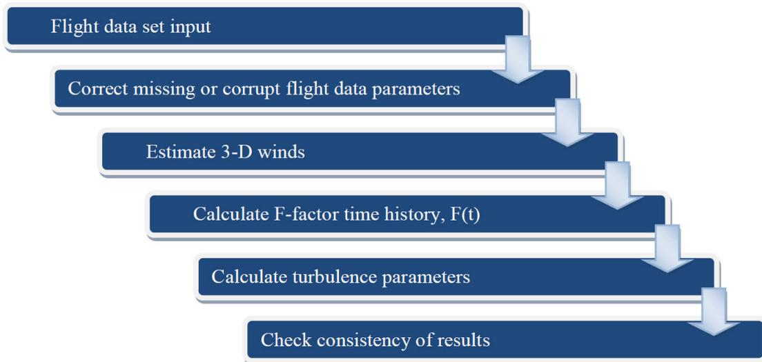
Figure 1: Flight Data Processing
