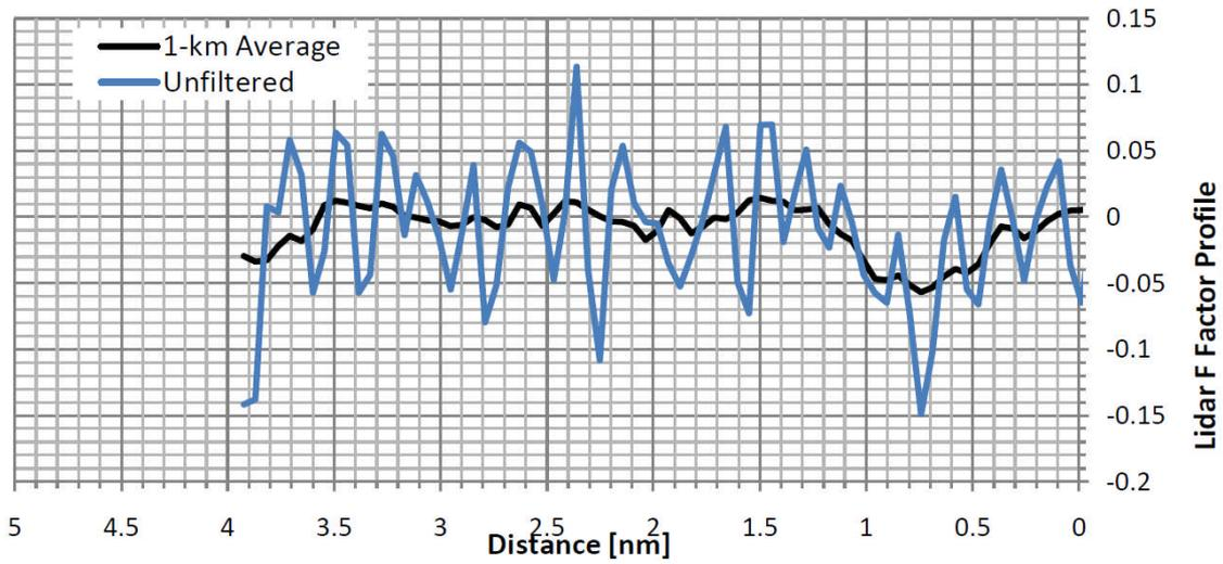
Figure 6: Unfiltered and 1-km averaged F-factor from LIDAR headwind profile
