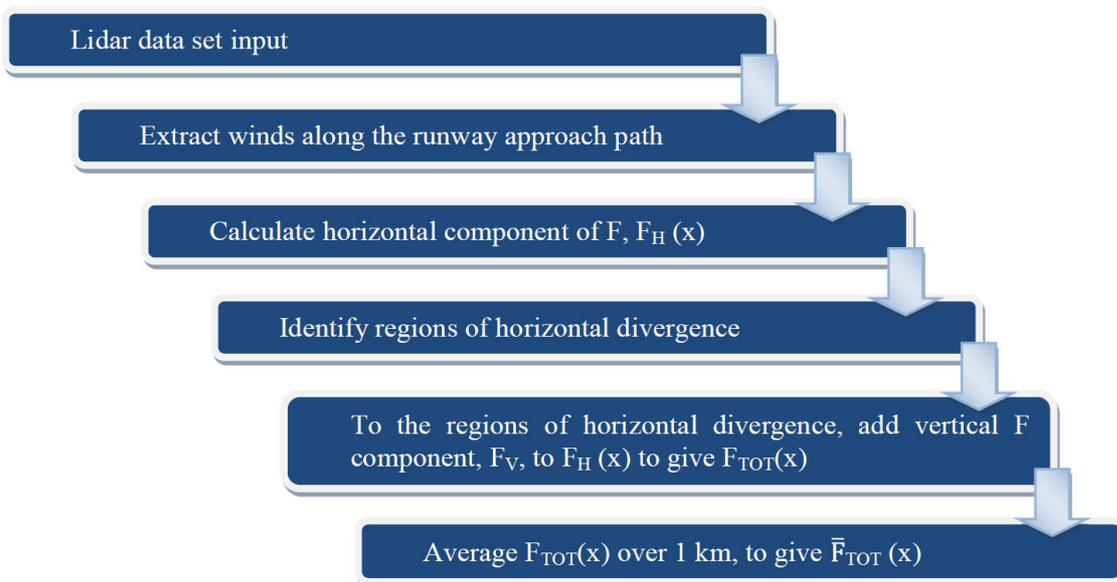
Figure 2: Lidar Data Processing
