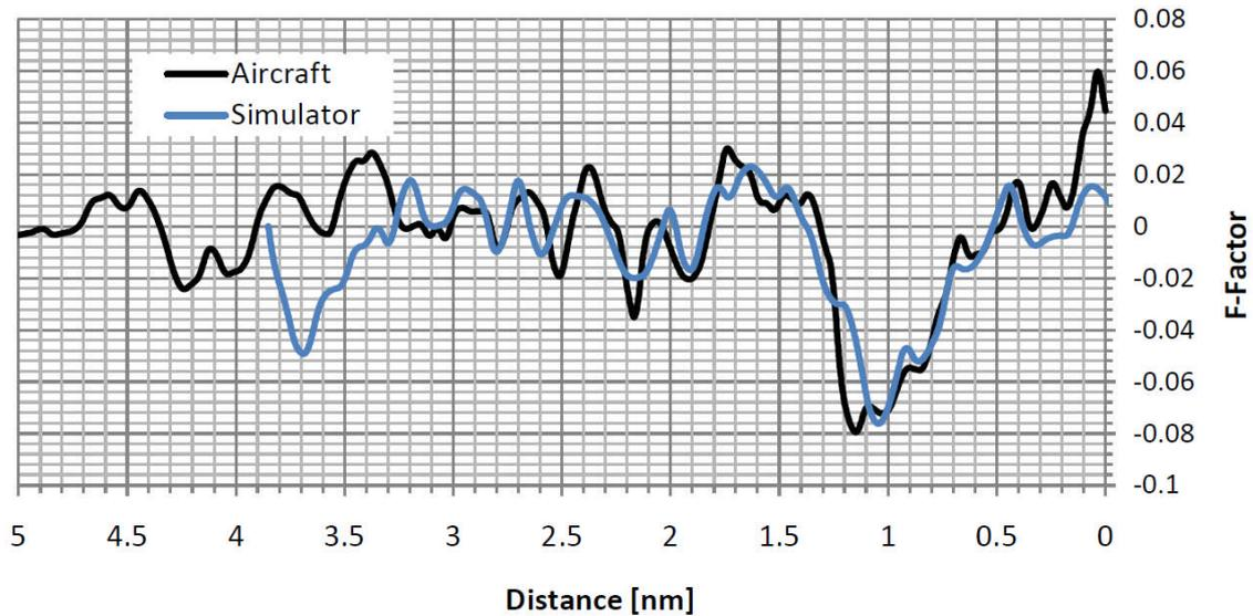
Figure 8: Aircraft and simulator F-factor comparison
