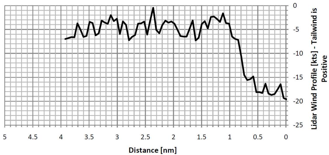
Figure 5: LIDAR headwind profile (distance from runway threshold)
