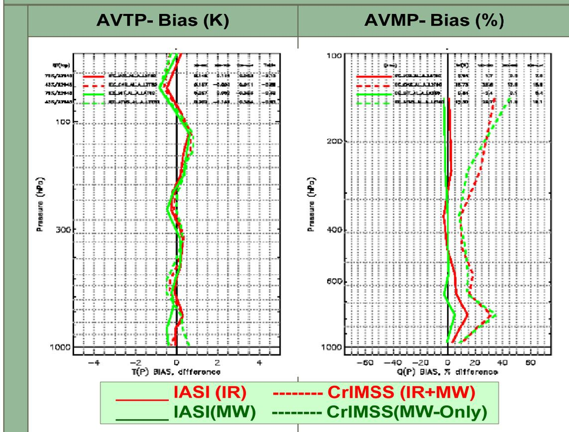
Figure 9b. NGAS-CrIMSS and IASI EDR Statistics with ECWMF analysis fields for the ocean-only cases. The CrIMSS AVTP product is quite comparable with the IASI EDR product. CrIMSS AVMP RMS difference for the middle and upper troposphere shows a little larger RMS difference compared with the IASI EDR product.
