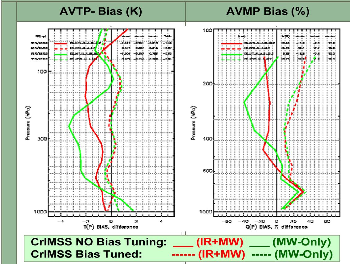
Figure 6. The CrIMSS AVTP and AVMP biases before and after the bias-tuning procedure. These figures reveal that the bias-tuning component implemented in the CrIMSS EDR code is critical for the EDR algorithm performance.
