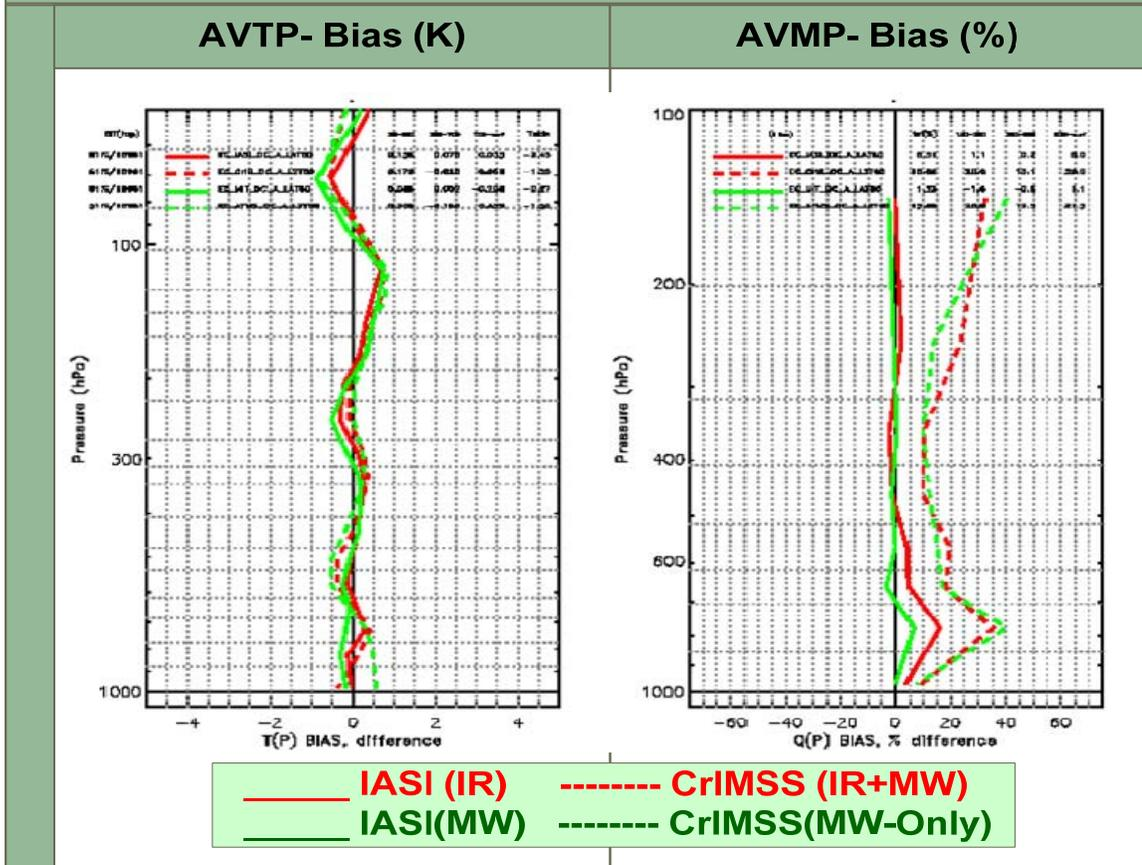
Figure 7b. AVTP and AVMP biases for NGAS-CrIMSS and IASI EDRs with reference to ECMWF analysis fields for the ocean-only cases. The CrIMSS AVTP biases show similar tendency to that of IASI EDR product. CrIMSS AVMP product shows a little larger wet bias with reference to ECMWF analysis fields. This requires further investigation.
