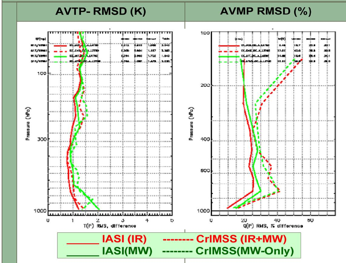
Figure 7a. AVTP and AVMP RMS differences for NGAS-CrIMSS and IASI EDRs with reference to ECWMA analysis fields for the ocean-only cases. The CrIMSS AVTP products from both the stages ('MW-only'; IR+MW') are quite comparable to the corresponding IASI EDR AVTP products. The CrIMSS AVMP RMS difference for the middle and upper troposphere shows a little larger RMS difference compared to the IASI AVMP product.
