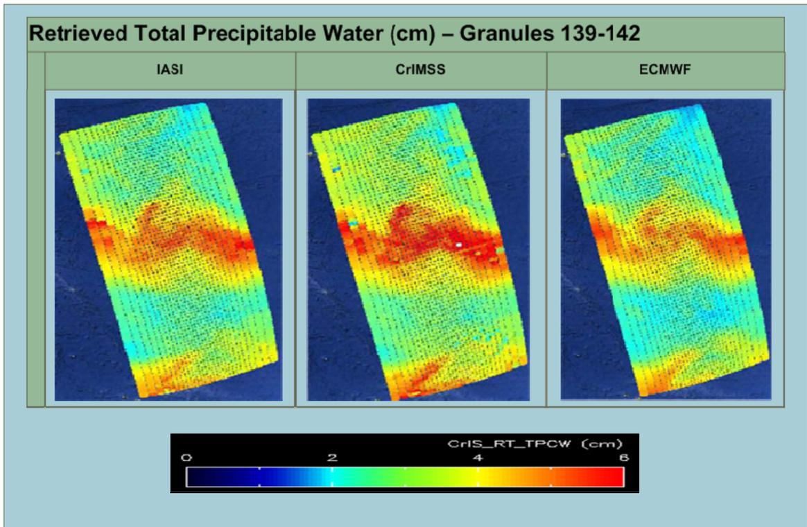
Figure 8. Comparison of Total Precipitable Water (TPW) derived from the NOAA-IASI EDRs, CrIMSS-EDRs and the ECMWF analysis fields for Granules 139-142 over the ocean (Figure 4). The figures reveal a slight overestimation of water vapor by the CrIMSS EDR algorithm in comparison to the ECWMF analysis fields, and rightly portrayed as a wet bias seen in Figure 7b for the CrIMSS AVMP.
