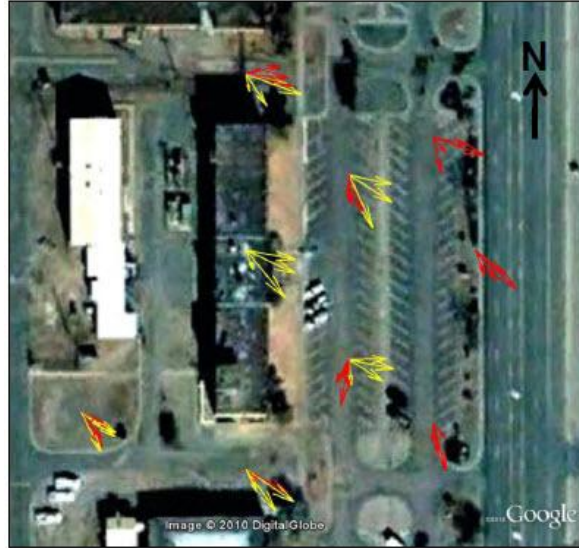
Figure 3. W07US low velocity, Northwest fetch case with a leeward, low level, northerly circulation. Yellow vectors are 10 m AGL; Red vectors are 2.5 m AGL.
