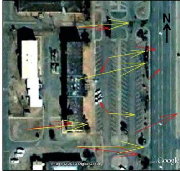
Figure 7. W07US high velocity, Westerly fetch case with a leeside, low level, center-convergence. Yellow vectors are 10 m AGL; Red vectors are 2.5 m AGL.
