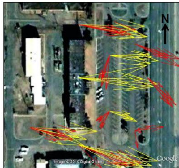
Figure 4. W07US high velocity, Northwest fetch case with a leeward, low level, north-northeasterly circulation. Yellow vectors are 10 m AGL; Red vectors are 2.5 m AGL.
